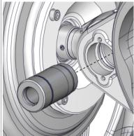
Press in the shaft using the dismantle and mounting tool, according to user instructions enclosed with the equipment.
