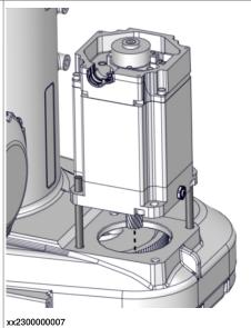
Whenever parting/mating motor and gearbox, the gears may be damaged if excessive force is used.
