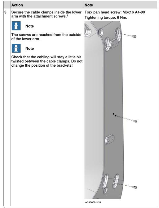
If the lower arm only has attachment holes for two cable clamps, either remove the third cable bracket from the spare part cable harness, or drill attachment holes in the lower arm. Contact ABB for more information.
