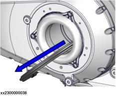
Removing the arm house cover including the cassette sealing
