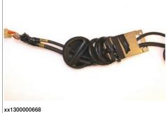
Run the cable harness through the cable guide and then into and through the upper arm tube.
