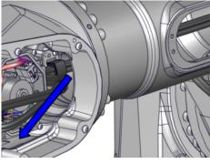
Refit the metal clamp axis-4, inside the arm Torx pan head screw: M6x16 A4-80 tube.
