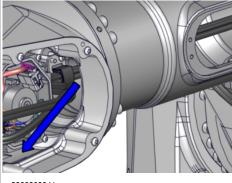
5 Refit the metal clamp axis-4, inside the arm Torx pan head screw: M6x16 A4-80 tube.
